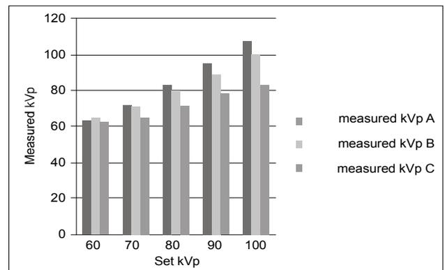
**Figure 2:** kVp variations compared for the different x-ray machines A - C. kVp affects the penetration of the x-rays. Variations at lower kVps would result in decreased x-ray penetration thereby increasing patient dose. Higher kVp variations would result in increased x-ray penetration thereby decreasing patient dose. However, this effect may affect the image quality leading to repeat exposure and indirectly increasing patient radiation dose.
