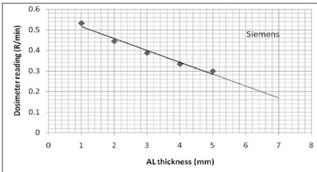
**Figure 4:** HVL graph for Siemens (x-ray unit B). This shows a HVL of about 5 mm at 80 kVp. The HVL should have a minimum of 2.3 mm Aluminium thickness at 80 kVp.<sup>19</sup>
