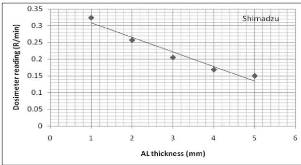
**Figure 3:** HVL graph for Shimadzu (x-ray unit A) and this shows a HVL of about 4.4 mm at 80 kVp. The HVL should have a minimum of 2.3 mm Aluminium thickness at 80 kVp.<sup>19</sup>
