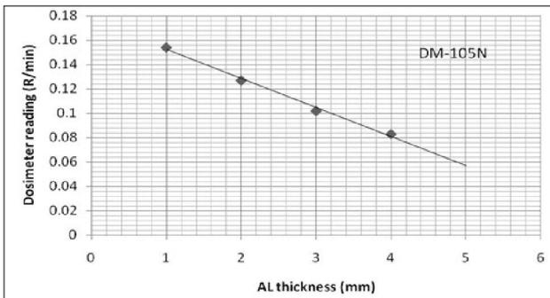
**Figure 5:** HVL graph for DM-105N (x-ray unit C). This shows that a HVL value of about 4 mm at 80 kVp. The HVL should have a minimum of 2.3 mm Aluminium thickness at 80 kVp.<sup>19</sup>
